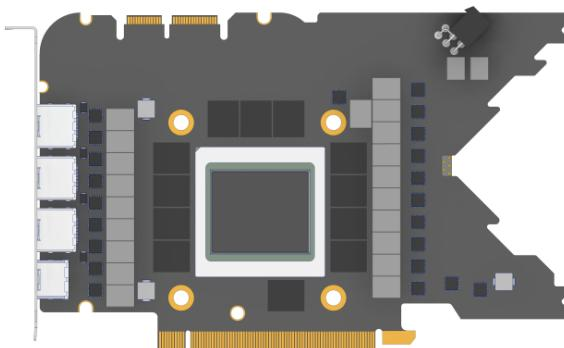
**EN** Put the hardware on an antistatic mat. Begin dismantling the original cooler. Depending on the structure of the cooler, remove the screws at the back of the card and carefully unhook the fan connector first. If the original cooler uses thermal glue, extreme care should be taken as you can easily damage parts. Pick up all the items carefully. Next, clean the hardware of thermal paste or pad residues with a solvent (e.g. isopropanol alcohol).
