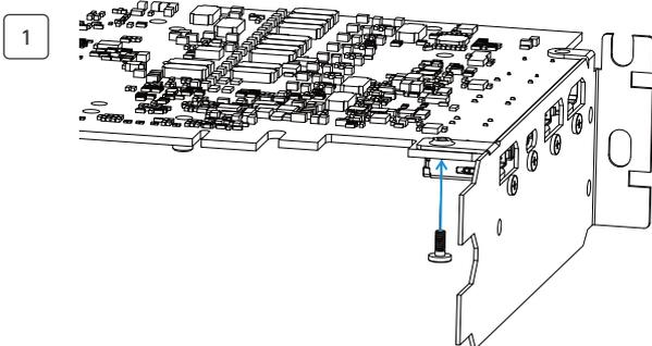
Use the original screws of the graphics card (1) and use the screws supplied in the accessories (2).
