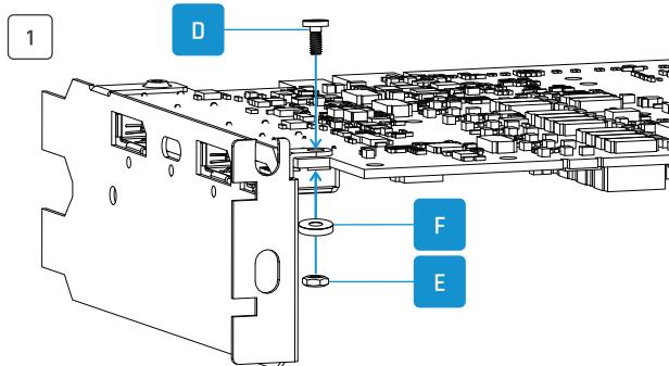
Use the screws supplied in the accessories (1) and the original screws of the graphics card (2).
