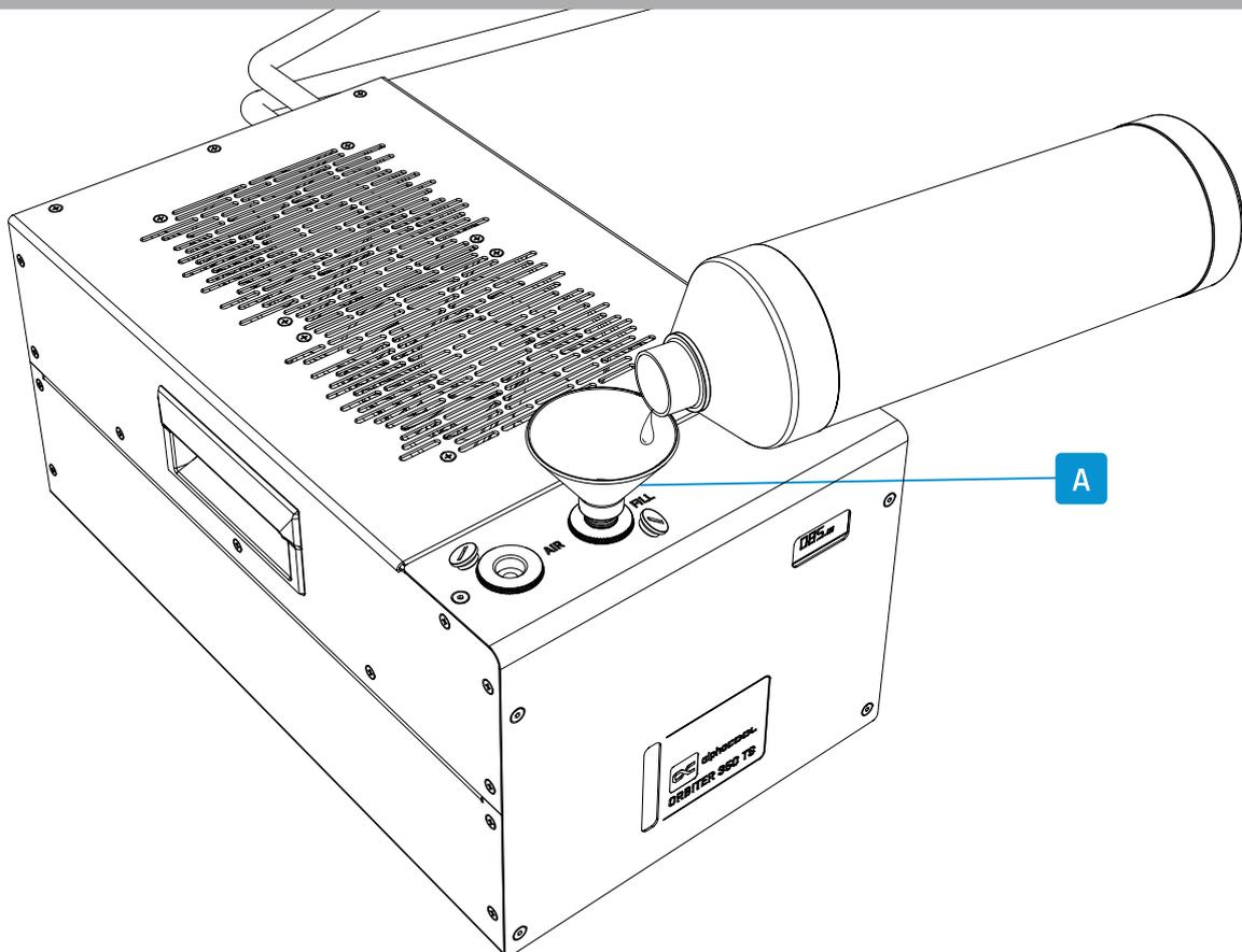
Do not operate the orbiter without coolant!
