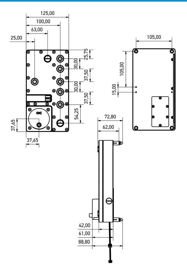
General tolerance: ± 0,25mm Dimension in millimeter
