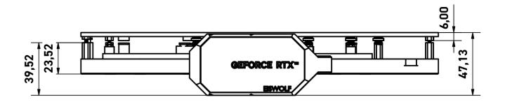
General tolerance:  $\pm$  0,25mm Dimension in millimeter
