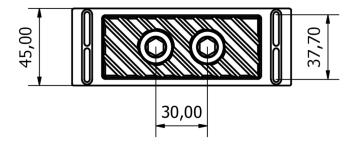
General tolerance: ± 0,25mm Dimension in millimeter
