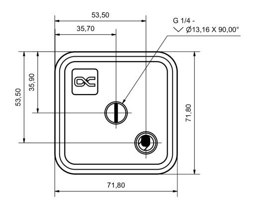
General tolerance: ± 0,25mm Dimension in millimeter
