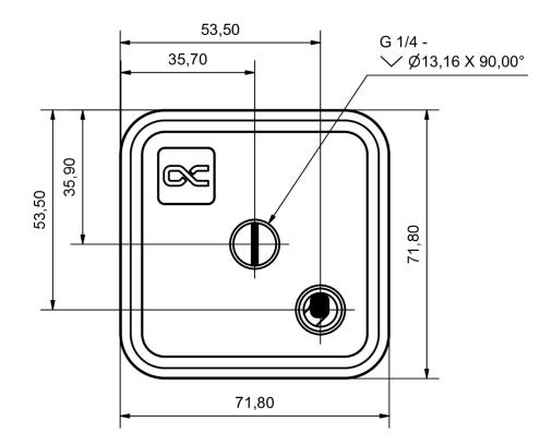
General tolerance:  $\pm$  0,25mm Dimension in millimeter
