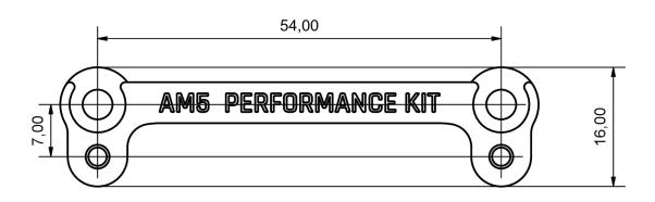
General tolerance:  $\pm$  0,25mm Dimension in millimeter
