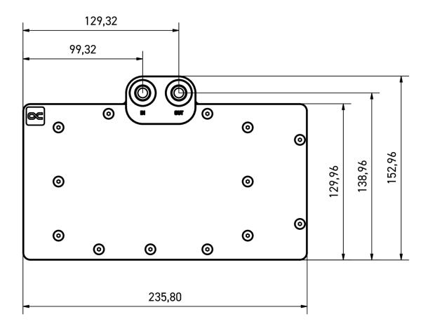
General tolerance: ± 0,25mm Dimension in millimeter
