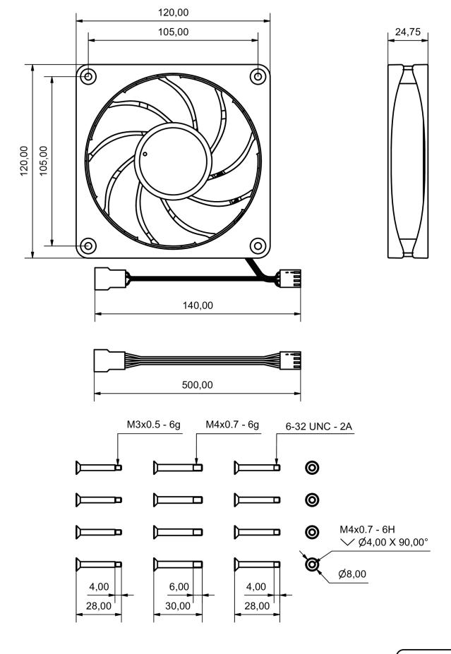
General tolerance: ± 0,25mm Dimension in millimeter
