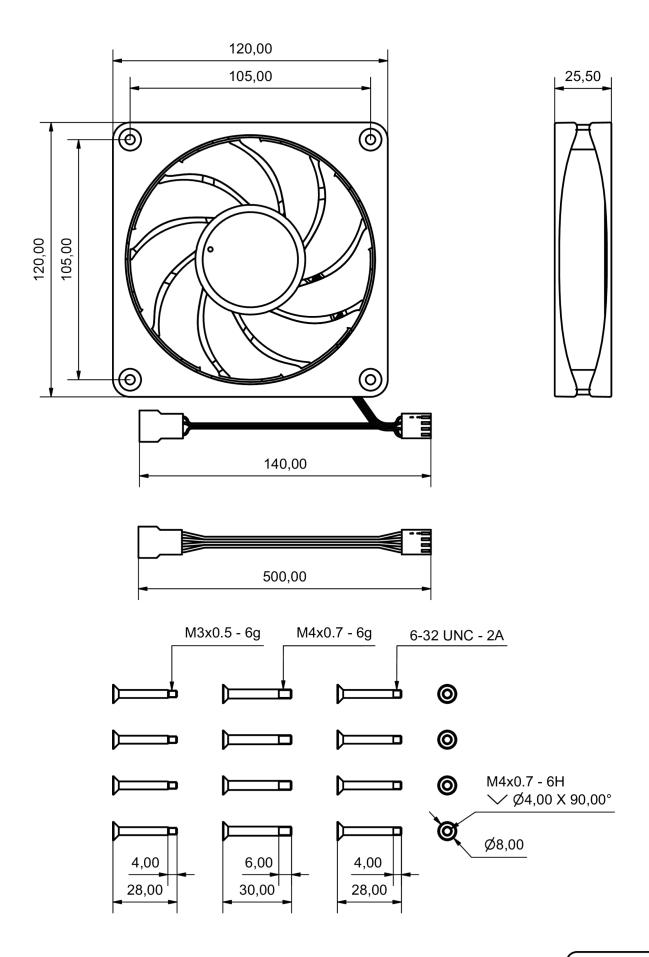
General tolerance: ± 0,25mm Dimension in millimeter
