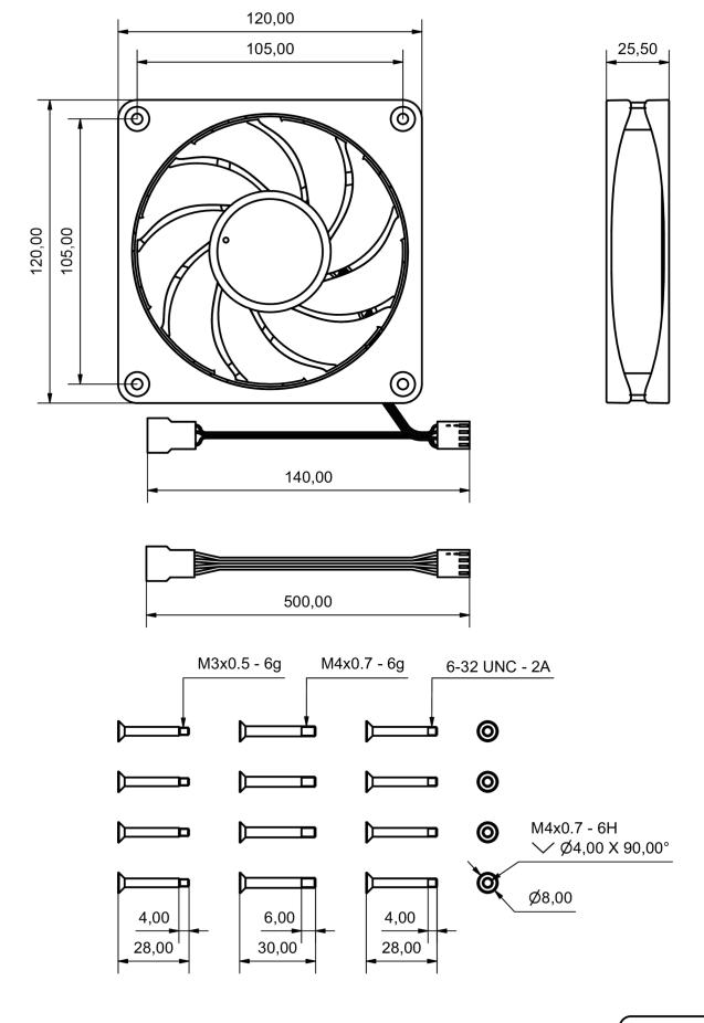
General tolerance: ± 0,25mm Dimension in millimeter
