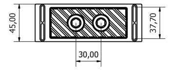
General tolerance: ± 0,25mm Dimension in millimeter
