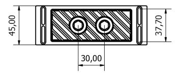
General tolerance: ± 0,25mm Dimension in millimeter
