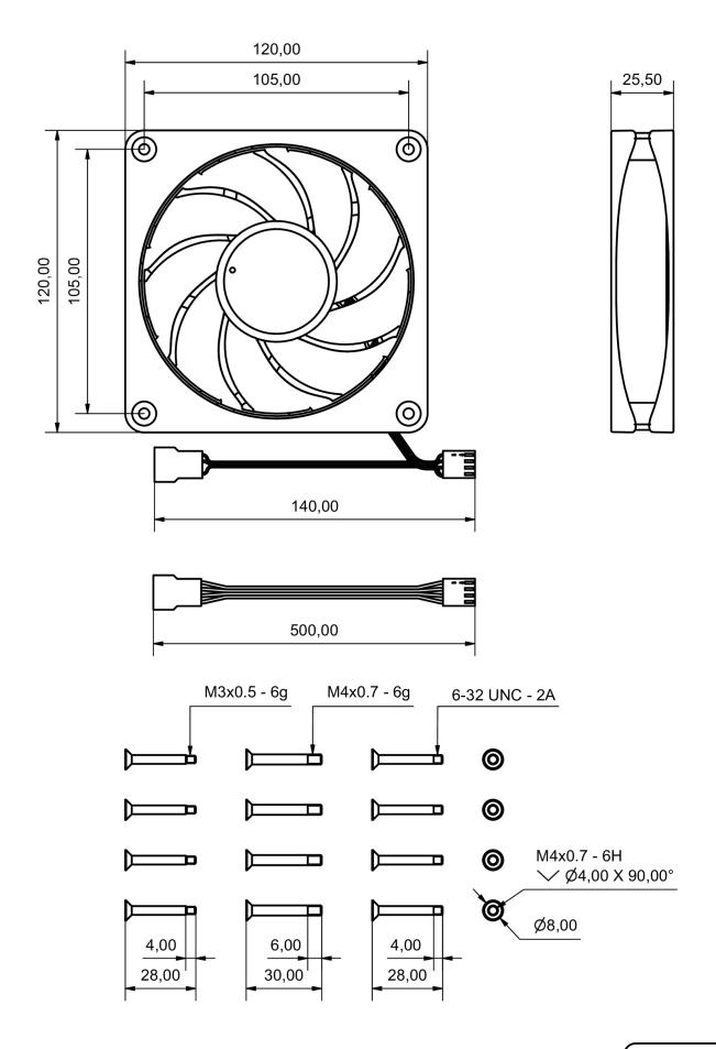
General tolerance: ± 0,25mm Dimension in millimeter
