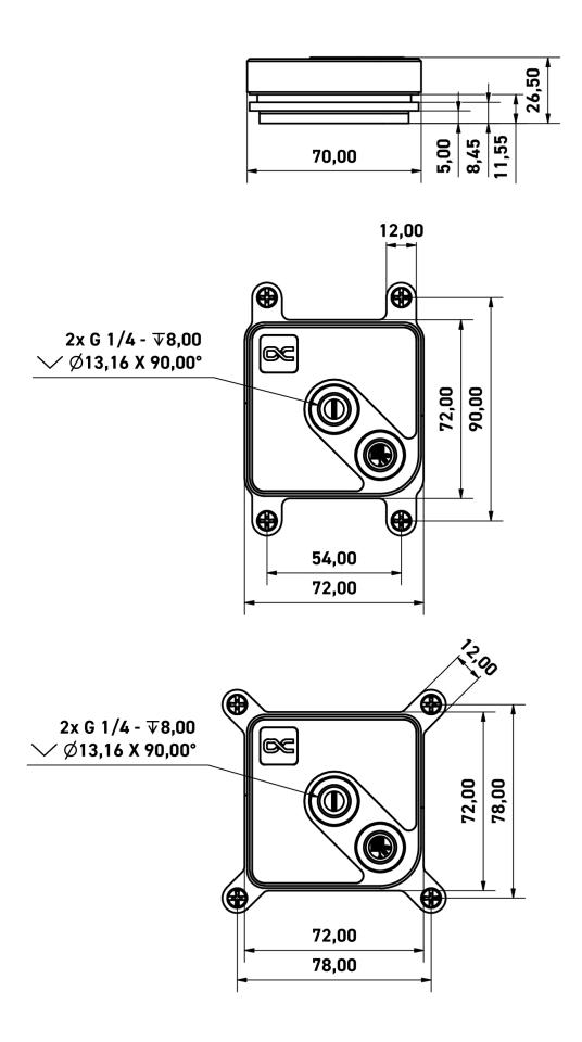
General tolerance: ± 0,25mm Dimension in millimeter
