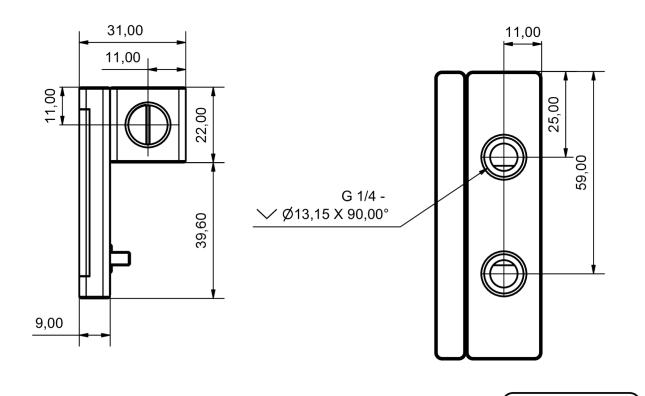
General tolerance: ± 0,25mm Dimension in millimeter
