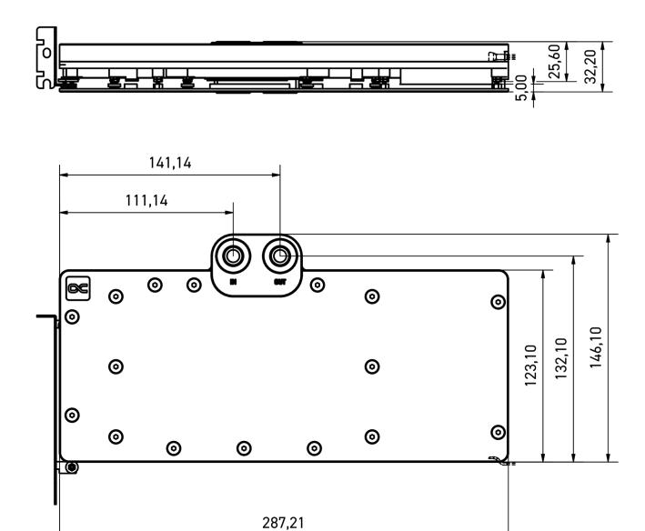
General tolerance: ± 0,25mm Dimension in millimeter
