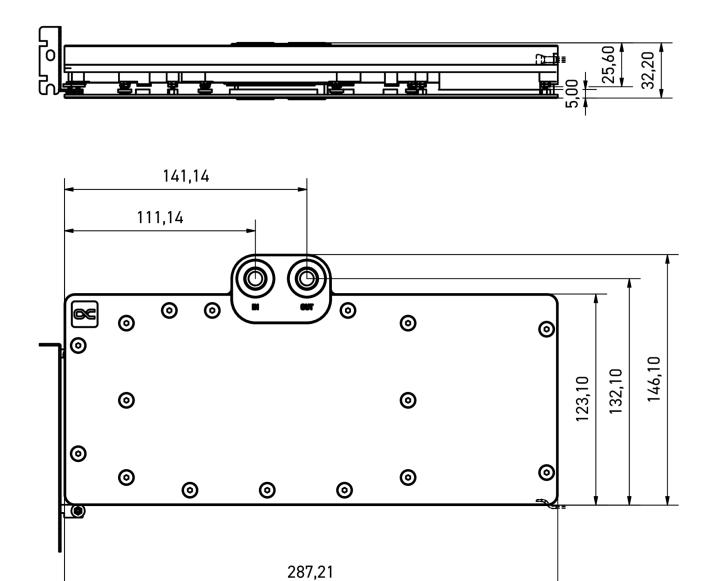
General tolerance: ± 0,25mm Dimension in millimeter
