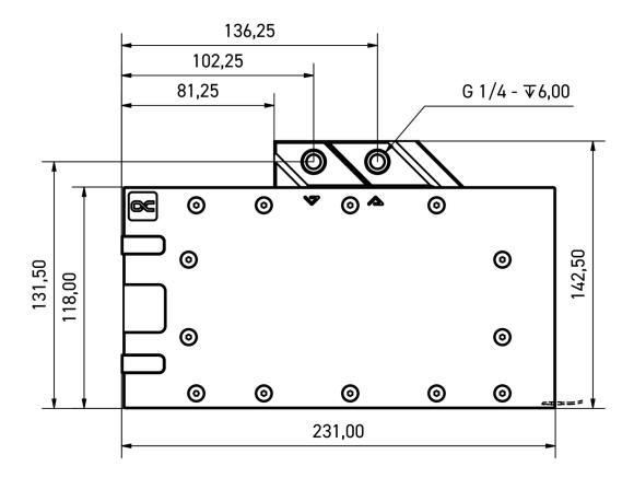
General tolerance: ± 0,25mm Dimension in millimeter
