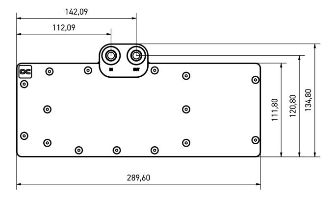
General tolerance: ± 0,25mm Dimension in millimeter
