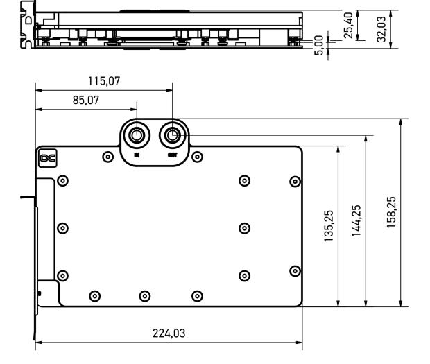
General tolerance: ± 0,25mm Dimension in millimeter
