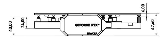
General tolerance:  $\pm$  0,25mm Dimension in millimeter
