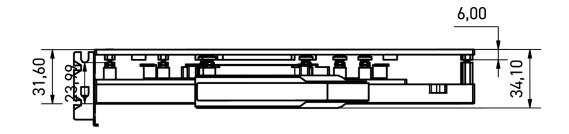
General tolerance: ± 0,25mm Dimension in millimeter
