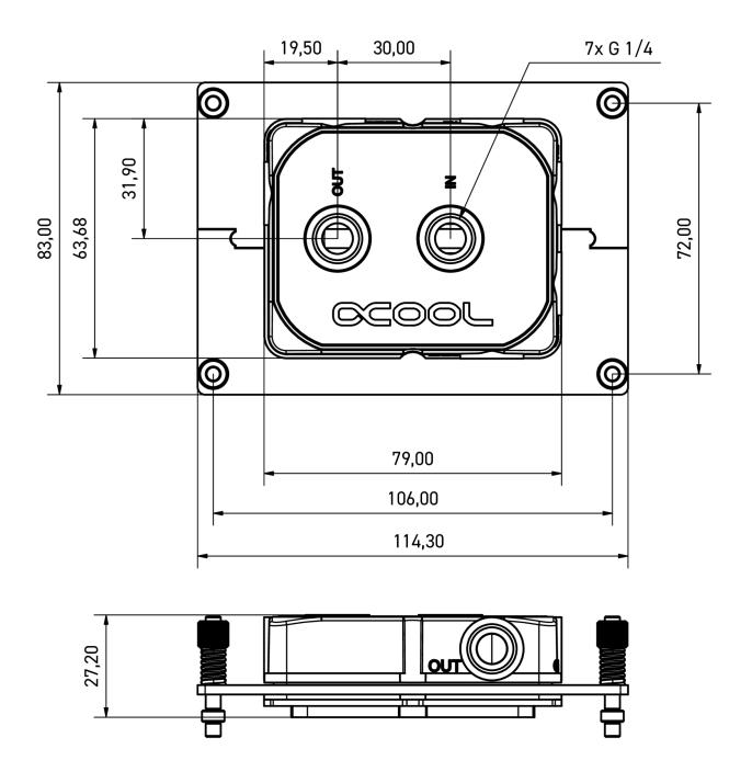
General tolerance: ± 0,25mm Dimension in millimeter
