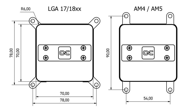
General tolerance: ± 0,25mm Dimension in millimeter
