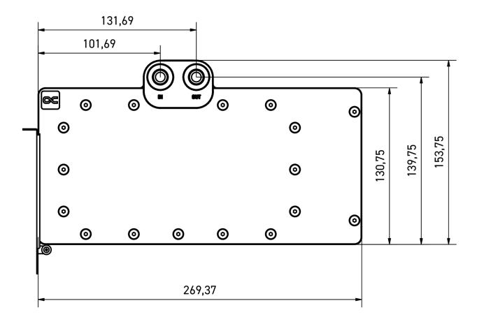
General tolerance: ± 0,25mm Dimension in millimeter
