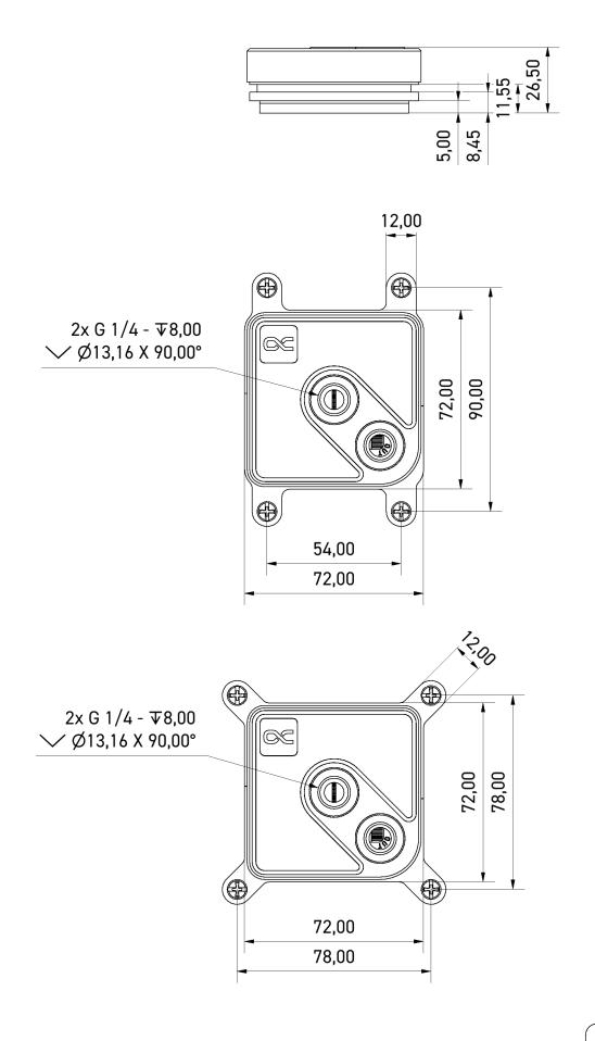
General tolerance: ± 0,25mm Dimension in millimeter
