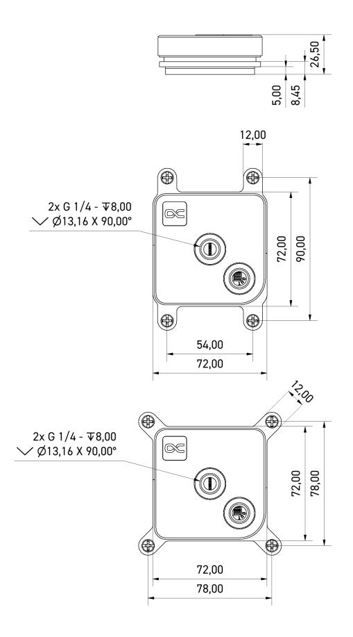
General tolerance: ± 0,25mm Dimension in millimeter
