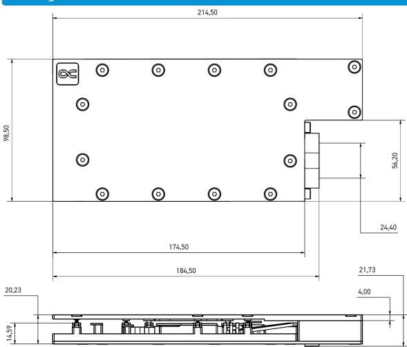
General tolerance: ± 0,25mm Dimension in millimeter
